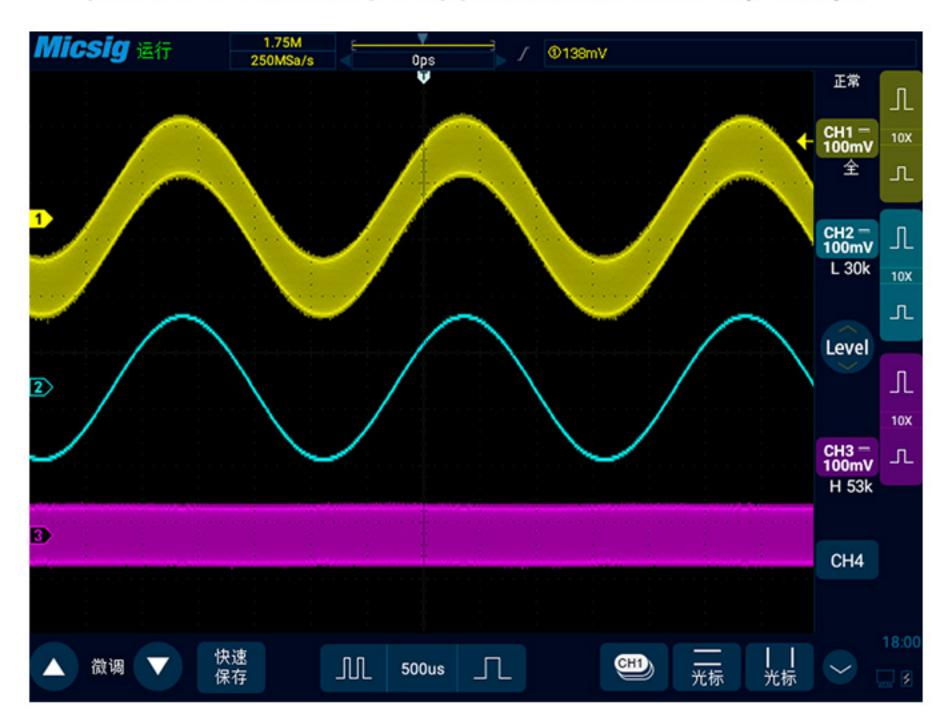
Most engineers focus on the details of a certain frequency band of a signal. Filtering out insignificant frequency to eliminate interference, realizes a better judgement of the signal
