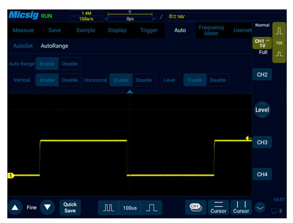
The scope can adjust the amplitude and horizontal time base in real time, ensures the waveform is always displayed with a suitable size on the screen, more convenient and accurate, avoids complicated manual adjustments.
