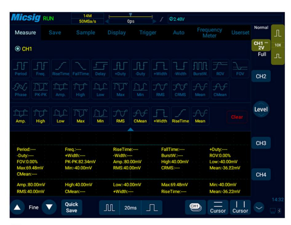
31 automatic measurements. Various automatic measurements can meet different measurement demand. It can be display all in one page.
