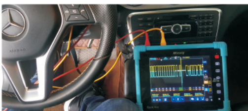
Power CAN bus communication
